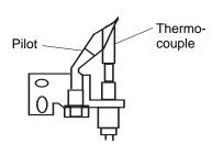
Figure 23 - Thermocouple and Pilot
